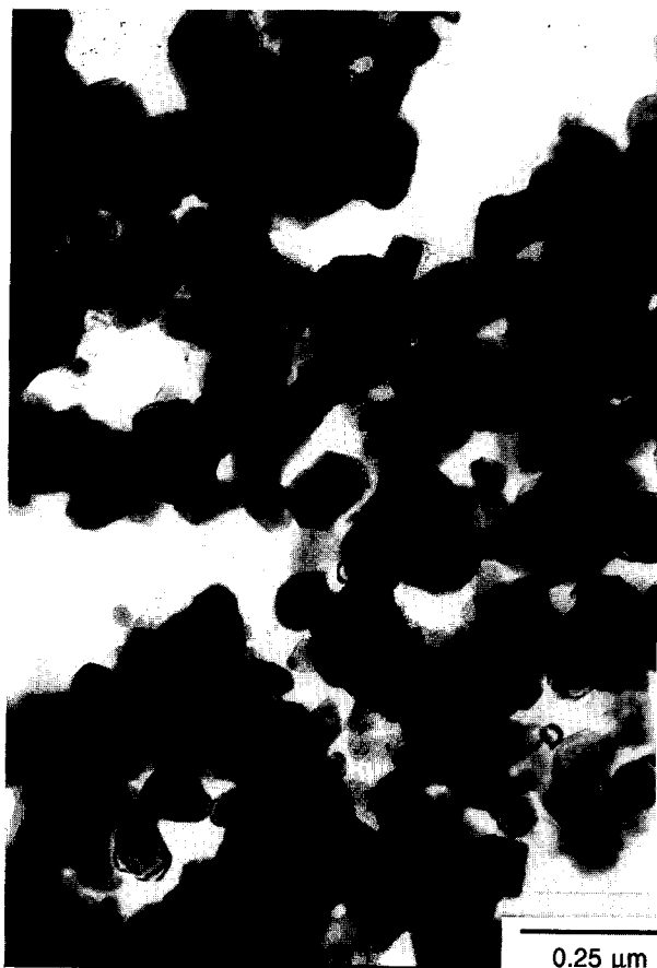
Fig. 8. TEM micrograph of TiC powder product synthesized at 1500°C for 4 h in flowing argon atmosphere.
